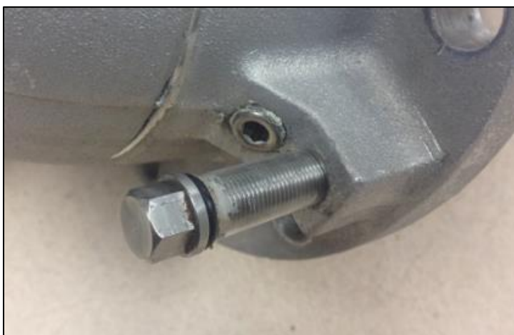
Figure 4: Valve after jack screw usage
