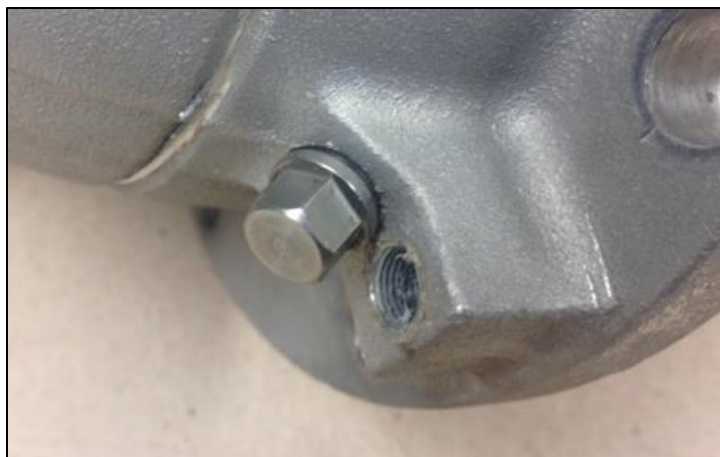
Figure 3: Fully installed jack screw
