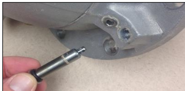
Figure 2: Hex head on end of jack screw
