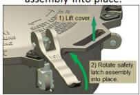
Hook first latch assembly into place using retention feature.
