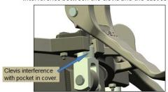
6 Lift cover slightly off collar seat to release safety latch assemblies.
