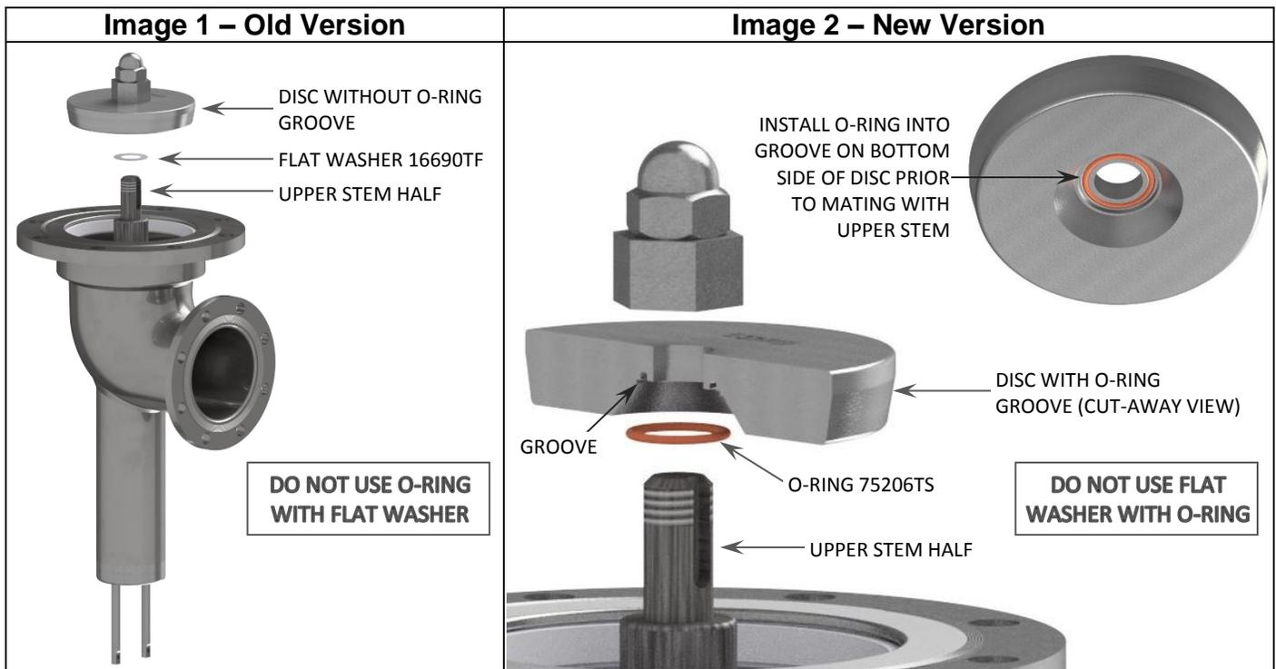
**Bulletin Instructions:** 75206TS O-ring is also used as the seal between the piston and piston holder. Rebuild kits will now include a second Tef-Sil O-ring (75206TS) to be used for the joint between the disc and upper stem, as highlighted above. Follow these guidelines for rebuild:
